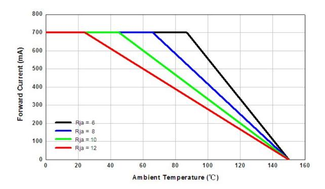
The junction temperature can be correlated to the thermal resistance between the junction and ambient (Rja) by the following equation.
